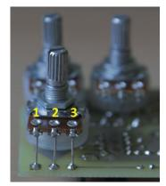
The pots are off board mounted via wires. For the numbering of the lugs see the picture.
