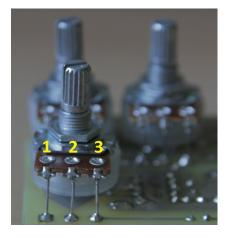
The pots are board mounted to the bottom of the board. The square pads mark the lug 1, for the numbering of the lugs see the picture. The switch is connected with off-board wires You can experiment with different opamp types. The original used the LM833, but I've found it sometimes too noisy. TL062 has helped in those cases a lot, but you can try some of the higher end Burr Brown opamps too, like the OPA2134.
