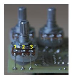
All pots are board mounted. The square pad marks the lug 1, for the numbering of the lugs see the picture.
