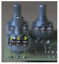
The pot is board mounted to the bottom of the board. The square pad marks lug 1, for the numbering of the lugs see the picture. Since the part number is quite low it is possible to build the effect into a 1590A box too. In this one you can experiment with different types of JFETs, neither the Mu-Amp, nor the buffer are too susceptible. I have used J201 and J202 with great success, but you can try 2N5457 or whatever you have access to. Pay attention to the pinout though, different types can vary.
