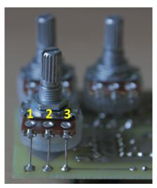
The pots are board mounted to the bottom of the board. The square pads mark the lug 1, for the
