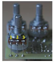
The pots are board mounted to the bottom of the board. The square pads mark the lug 1, for the numbering of the lugs see the picture. The smaller version has simple pads for connecting the pots with wires, this one can even be built into a 1590A enclosure. The numbering is the same as on the picture.
