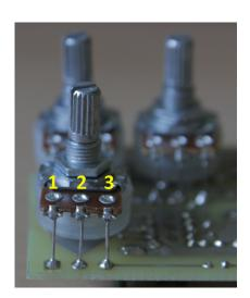
The pots are board mounted to the bottom of the board. The square pads mark the lug 1, for the numbering of the lugs see the picture. Since the part number is quite low it is possible to build the effect into a 1590A box too. That version however has simple pads for connecting the pots with wires. The numbering is the same as on the picture.
