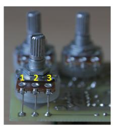
The Tone pot is mounted to the bottom of the board. The square pad marks the lug 1, for the numbering of the lugs see the picture. The Volume and Sustain pots are mounted off-board with wires.
