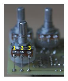
The pots are board mounted to the bottom of the board. The square pads mark the lug 1, for the numbering of the lugs see the picture. The switch is connected with wires and goes beneath the PCB. Make sure you leave enough space between the board and the switch to avoid shorting the circuit. I usually cut back the switch lugs and put a thicker double sided foam tape under the switch.
