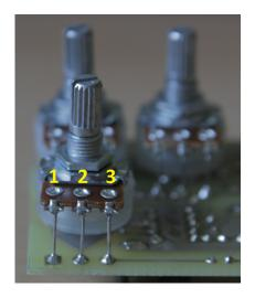
The pots are board mounted to the bottom of the board. The square pads mark the lug 1, for the numbering of the lugs see the picture.
