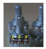
On the large layout all pots are board mounted. The square pad marks the lug 1, for the numbering of the lugs see the picture. The smaller layout uses off-board wiring for all pots.
