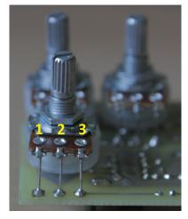
The Crunch and Volume pots are board mounted to the bottom of the board, the Tone pot has only the solder pads, connect it with wires. The square pads mark the lug 1, for the numbering of the lugs see the picture.
