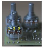
The pots are board mounted to the bottom of the board. The square pads mark the lug 1, for the numbering of the lugs see the picture.
