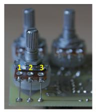
The pots are board mounted to the bottom of the board. The square pads mark the lug 1, for the numbering of the lugs see the picture. The original has a DPDT ON/ON/ON three position switch for the FCV control. The schematic and the layout are created to use this, but if you (like me) want to rather separate the clipping switch and the feedback switch, then you can use a simple SPST for the feedback and an SPDT ON/OFF/ON three position switch for the clipping. For further notes see the schematic.
