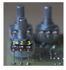
The pots are board mounted to the bottom of the board. The square pads mark the lug 1, for the numbering of the lugs see the picture. In the documentation found on <u>GCI</u> there is detailed description on how the effect works, there are suggestions too for mods even for the unusual EQ section taken from the DOD FX10 effect. My only additional suggestion for mods is that I would rather use a linear pot for Distortion.
