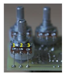
The pots are board mounted to the bottom of the board. The square pads mark the lug 1, for the numbering of the lugs see the picture. Since the part number is quite low it is possible to build the effect into a 1590A box too, but then the five pots will not fit. In that version I have omitted the Fat control and the 10nF C2 cap and used the 10uF C3 cap only since I've found that most of the time I'm using the effect with the Fat pot maxed out anyway.
