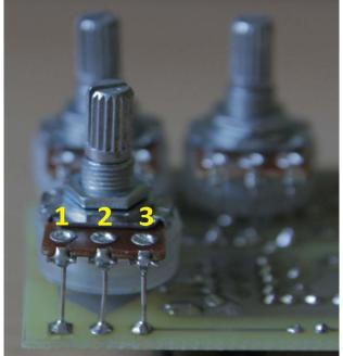
The pots are board mounted to the bottom of the board. The square pads mark the lug 1, for the numbering of the lugs see the picture.
