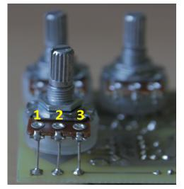
The Volume and Gain pots are board mounted and the Tone pot is connected off-board with wires on the large layout. The square pad marks the lug 1, for the numbering of the lugs see the picture. The smaller layout uses off-board wiring for all pots.
