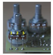
The pots are board mounted to the bottom of the board. The square pads mark the lug 1, for the numbering of the lugs see the picture. The switch is off-board mounted with wires. Due to the small size of the board it might be possible to squeeze it into a small 1590A box, but then low profile jack outlets and electrolytic caps and 9mm pots are a must. Also in this case you can't mount the pots on the board, they need to be mounted off-board with wires then.
