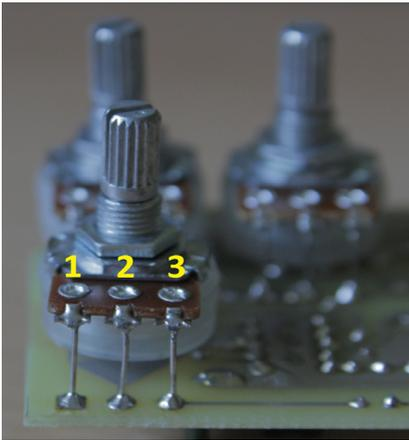
The pots are board mounted to the bottom of the board. The square pads mark the lug 1, for the numbering of the lugs see the picture. In the 1590A versions the pots are off-board mounted and connect to the board with wires. The lug numbering is the same. The switches in the drdFX250+ are also off-board mounted with wires.
